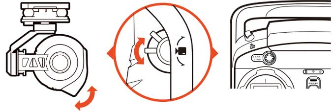
**QUICK TIP:** There's an adjustable counterbalance located on the rear of the CGO2+. This counterbalance has been adjusted at the factory to provide the best balance and performance overall so typically it should **NOT** need to be adjusted. However, if you find that the CGO2+ is making any 'buzzing' sounds while powered on, carefully twist the counterbalance in or out until the sound stops in order to achieve the best balance, performance and photo/video quality.
